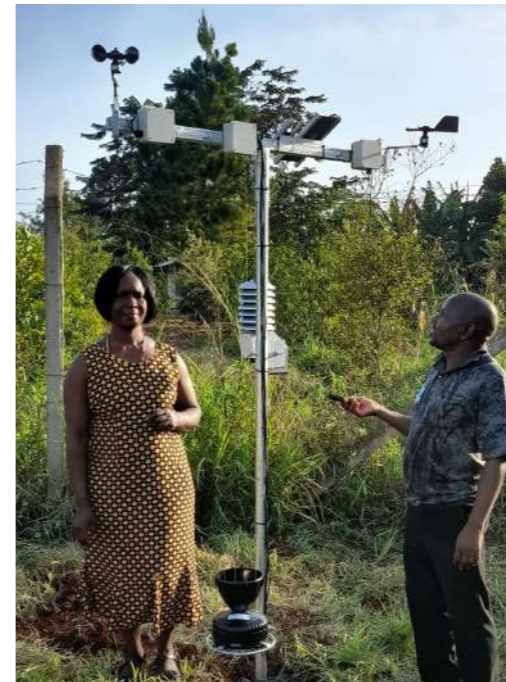
An installed AWS at Iganda Secondary School in Iganda district, Eastern Uganda
